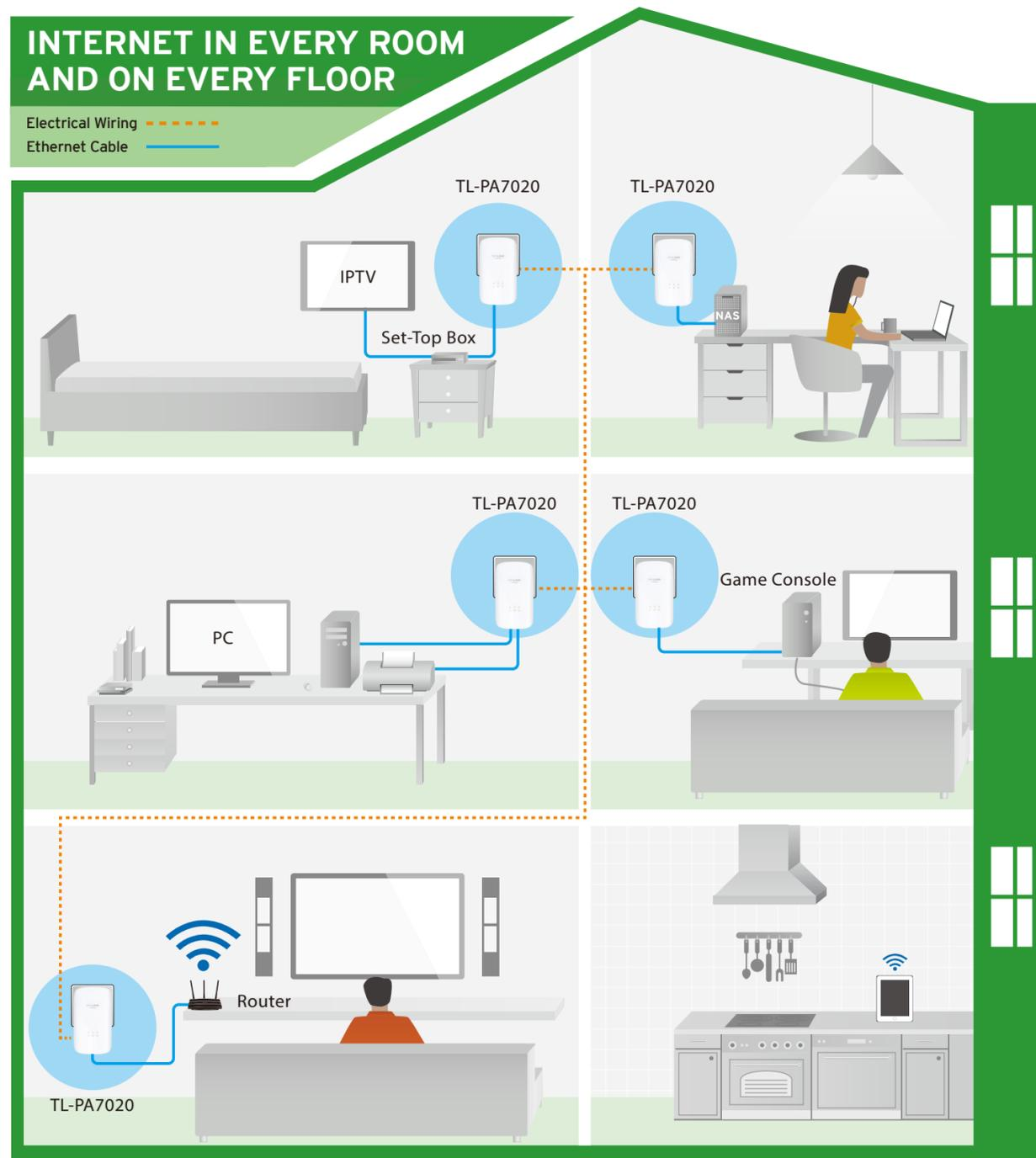
Note: The Powerline Adapters need to be connected to the same electrical circuit.
