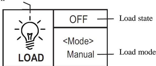
○,1. If the characters displayed on top of "<Mode>" are "ON", it indicates that the load is switched on, and "OFF" indicates the load is switched off.
