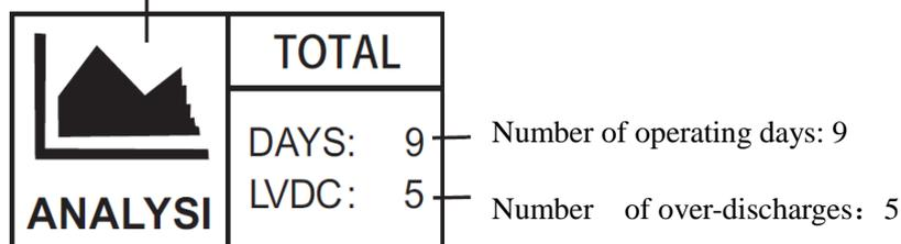
Including total charging amp-hrs, total discharging amp-hrs, total power consumption, numbers of operating days, over-discharges and full-charges
