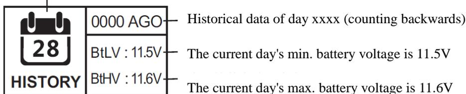
(Historical data including: the current day's min. battery voltage, the current day's max. battery voltage, the current
