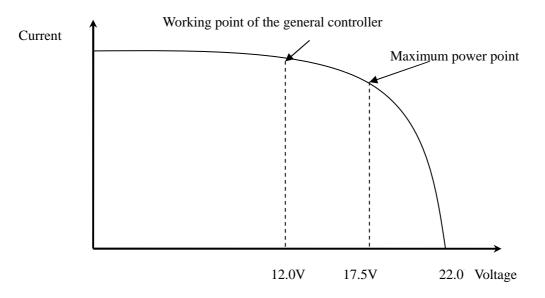
As a charging stage, MPPT can't be used alone. It must be combined with ascending charge, floating charge, equalizing charge to complete the battery charge.
