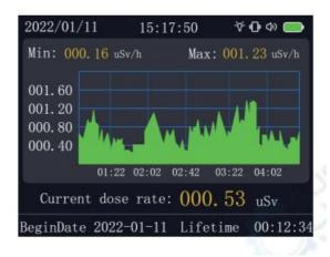
Press the left and right keys to switch to the waveform detection page as follows:
