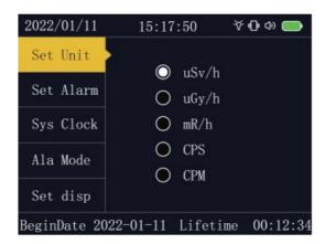
Press the right button to enter the lower level to set five measurement units:
