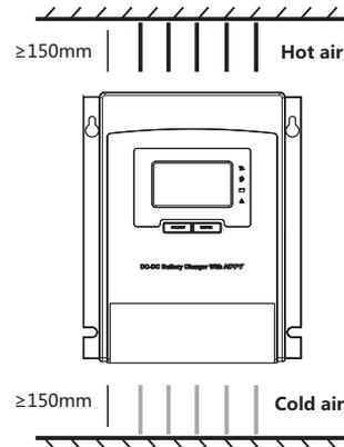
Fig. 4-1 Installation and Heat Dissipation
