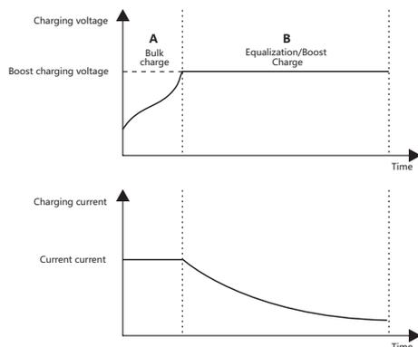
Fig. 1-6 Schematic Diagram of Lithium Battery Charging Stage
