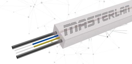
Masterlan MDIC is micro drop fiber optic cable suitable for any kind of use whether indoor or outdoor. It's outer jacket is low smoke, halogen free and UV stable to ensure great overall performance. Cable consist of 2 FRP strength members to protect fibers from mechanical damage. Quality materials provide easy use and handling. Used optical fibers are Corning (G.657.A1). There are two colours option, black and white.
