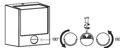
Adjust the sensor **sensitivity** by turning the dial on the left side.
