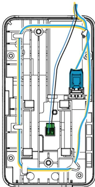
**Step 6** Secure the AP to the mounting bracket and tighten the screw on the side.
