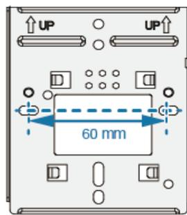
2. Use a 6 mm drill bit to drill 40 mm to 45 mm deep holes in the drilling positions. Hammer the expansion tubes into the holes until the expansion tubes are completely embedded into the wall.
