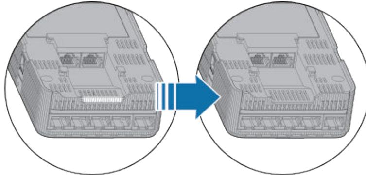
7. Tighten an M3x4 crosshead screw into the device to prevent the device from dropping. If the anti-theft function is required, tighten an M3x4 torx screw (instead of an M3x4 crosshead screw) into the device using a T9 torx security screwdriver. The tightening torques of the two screw types are both 0.15 N·m.
