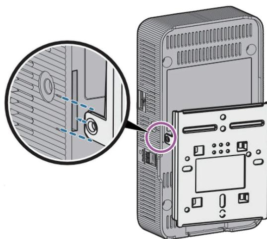
5. Align the four grooves on the bottom cover of the device with the upper ends of the clips on the mounting bracket. Slide the device downward to hang it on the mounting bracket.
