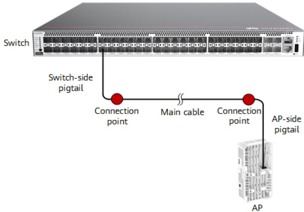
For details about the requirements for routing a hybrid cable, see [13.2.5.1 Requirements for Routing the Main Cable](#). The hybrid cable can be deployed using the optical-electrical separation solution or optical-electrical integration solution.
