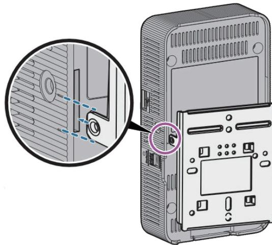
6. Align the four grooves on the bottom cover of the device with the upper ends of the clips on the mounting bracket. Slide the device downward to hang it on the mounting bracket.
