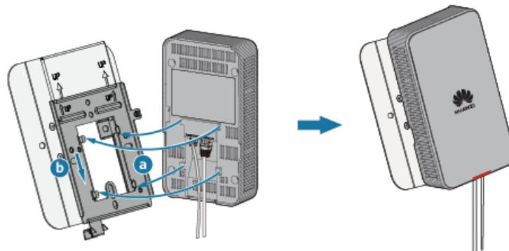
5. Tighten an M3x4 crosshead screw into the device to prevent the device from dropping. If the anti-theft function is required, tighten an M3x4 torx screw (instead of an M3x4 crosshead screw) into the device using a T9 torx security screwdriver. The tightening torques of the two screw types are both 0.15 N·m.
