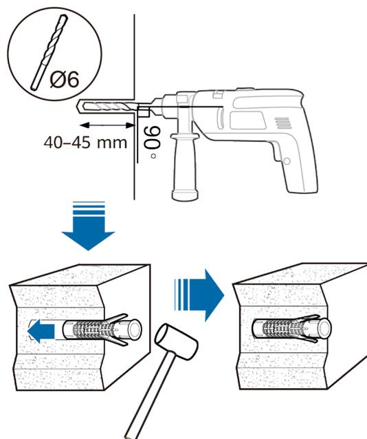
3. Fix the mounting bracket to the wall, and use the Phillips screwdriver to fasten two expansion screws into the expansion tubes to secure the mounting bracket to the wall.
