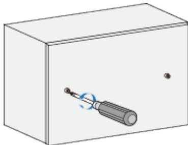
2. Secure the mounting bracket (118 mm) to the junction box using two M4x25 screws.
