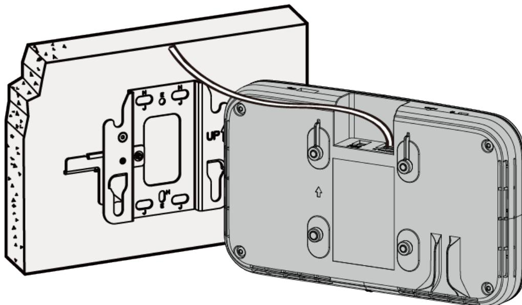
5. Align the four rubber feet at the rear of the AP with the installation holes on the mounting bracket, and fasten the device as shown in the figure. When you hear a click, the AP is secured to the lock position.
