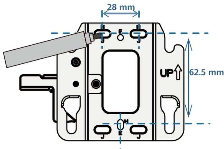
2. Use a 6 mm drill bit to drill 40 mm to 45 mm deep holes in the drilling positions. Hammer the expansion tubes into the holes until the expansion tubes are completely embedded into the wall.
