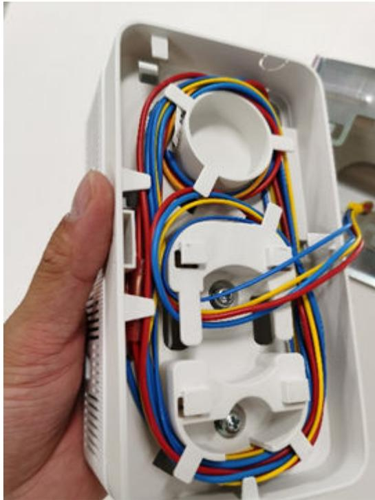
**Step 6** Secure the AP to the mounting bracket by using the two grooves on the side and the guide rail on the rear of the fiber management tray, and tighten the screws on the side.
