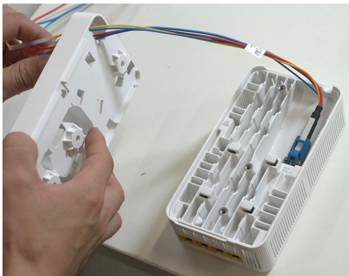
**Step 4** Use three M4x12 screws to secure the fiber management tray to the rear of the AP.
