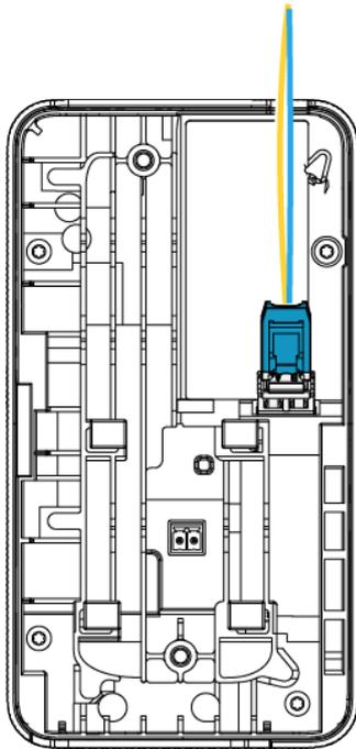
**Step 4** Coil the optical fiber counterclockwise to a proper length according to the arrow on the bottom shell.
