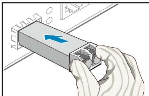
5. Check that the optical module is installed correctly. Keep the release handle closed and try pulling the optical module by pressing the optical module with your forefinger and thumb to see if the optical module can be removed.
