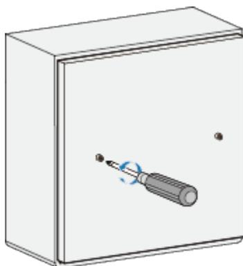
2. Secure the mounting bracket to the junction box using two M4x25 screws.
