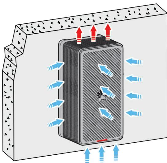
Reserve at least 200 mm clearance around an AP. In junction box mounting scenarios, ensure that the AP is at least 200 mm high from the floor. In other mounting scenarios, it is recommended that an AP be mounted 2.5 m to 3.5 m from off the floor. [Figure 3-37](#) shows space requirements. In wall or junction box mounting scenarios, 200 mm or a larger space is recommended between the AP and ceiling to achieve better heat dissipation.
