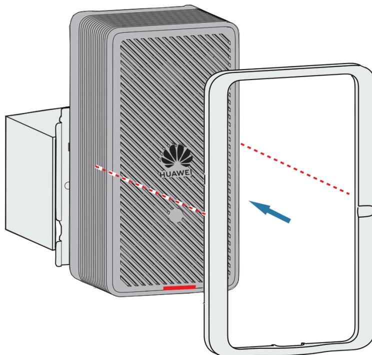
6. Tighten an M3x4 crosshead screw into the device to prevent the device from dropping. If the anti-theft function is required, tighten an M3x4 torx screw (instead of an M3x4 crosshead screw) into the device using a T9 torx security screwdriver. The tightening torques of the two screw types are both 0.15 N·m.
