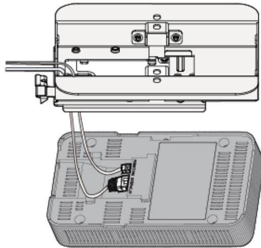
4. Align the grooves on the bottom cover of the device with the upper ends of the clips on the mounting bracket. When the device reaches the right place, the spring clip on the mounting bracket automatically falls back to secure the device.
