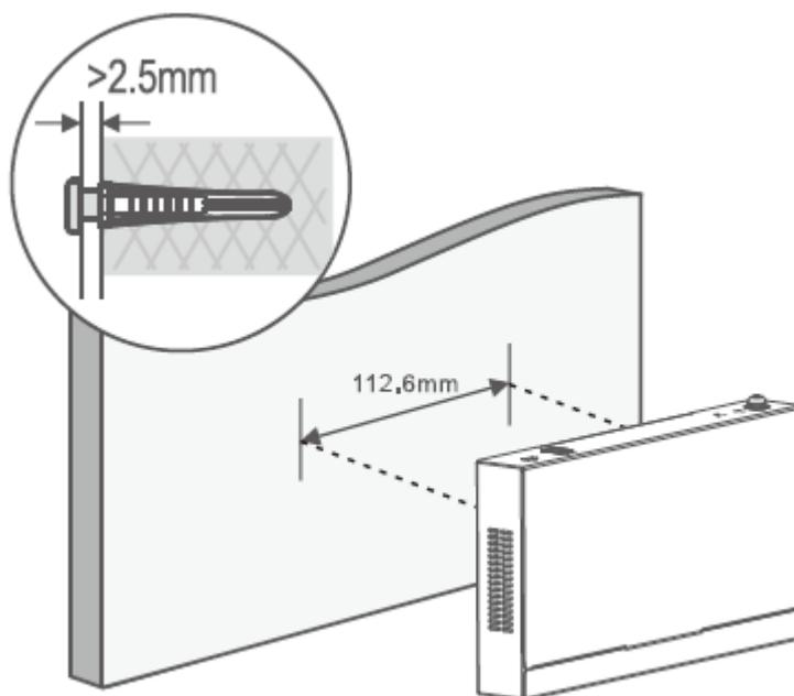
Note: When the device is mounted on a wall, it is only suitable to be mounted on a concrete or non-flammable surface.
