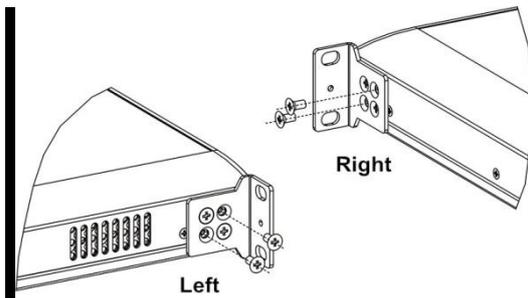
Figure 3-3 Securing Mounting Brackets
