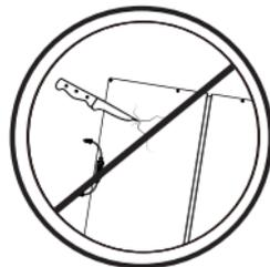
Behaviors above that damage the solar panel, will cause the cell inside the solar panel to crack and efficiency drop, or even unusable. The free warranty period does not cover damage resulting from improper use of the product.
