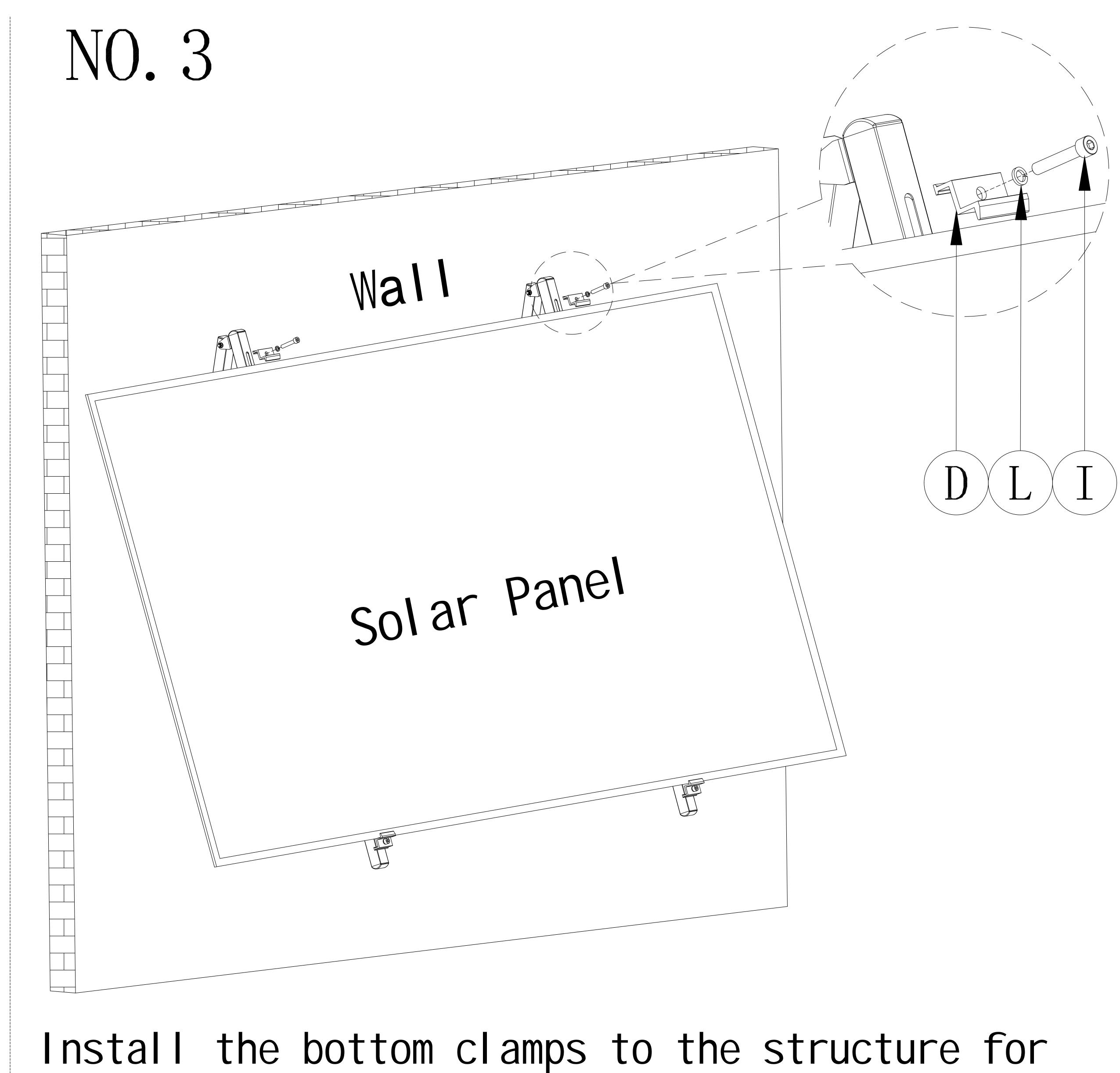
Install the bottom clamps to the structure for bottom to fix the whole mount on the wall
