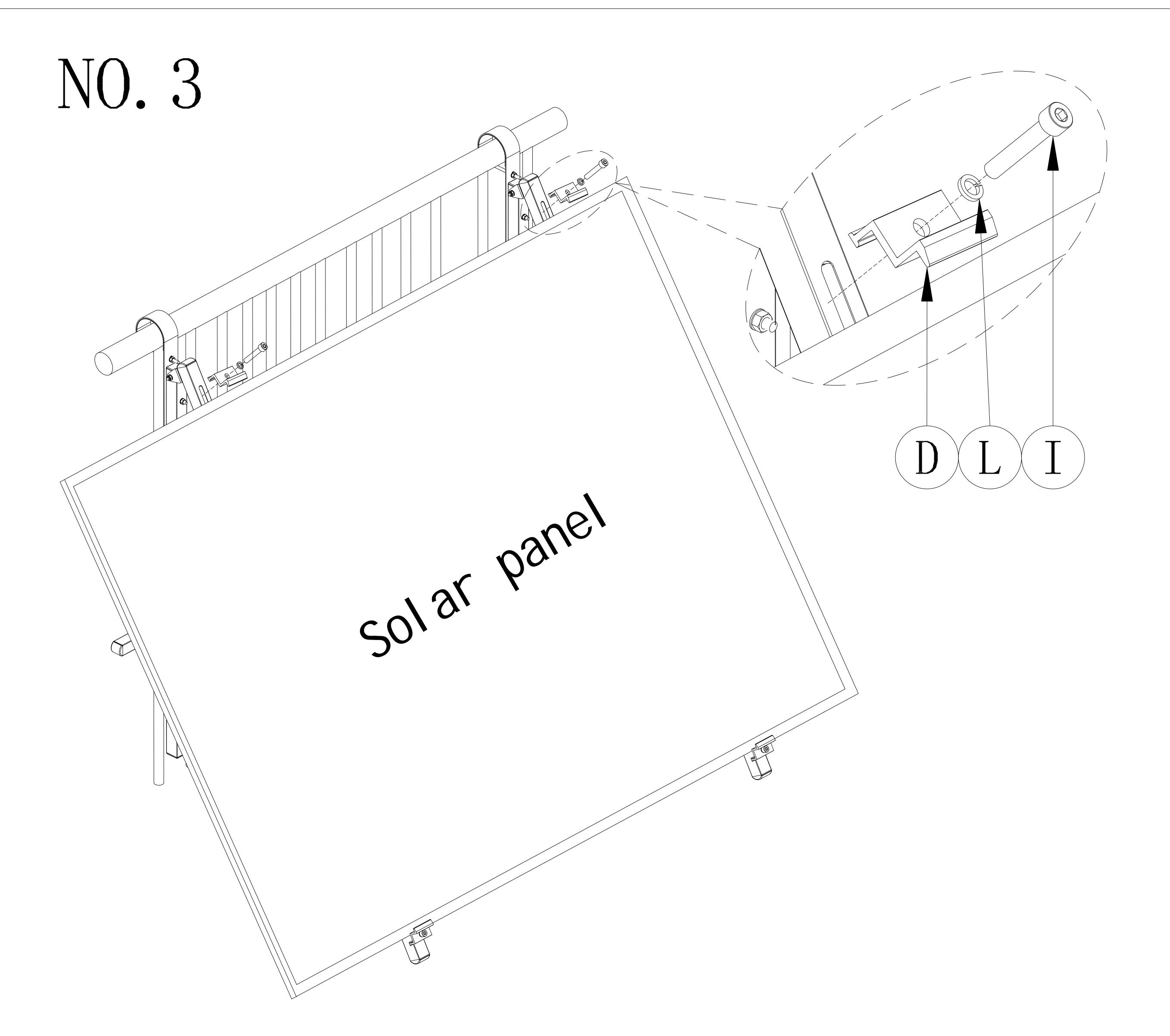
Before installing the hook, remove the hook screws and then install the hook to the bracket
