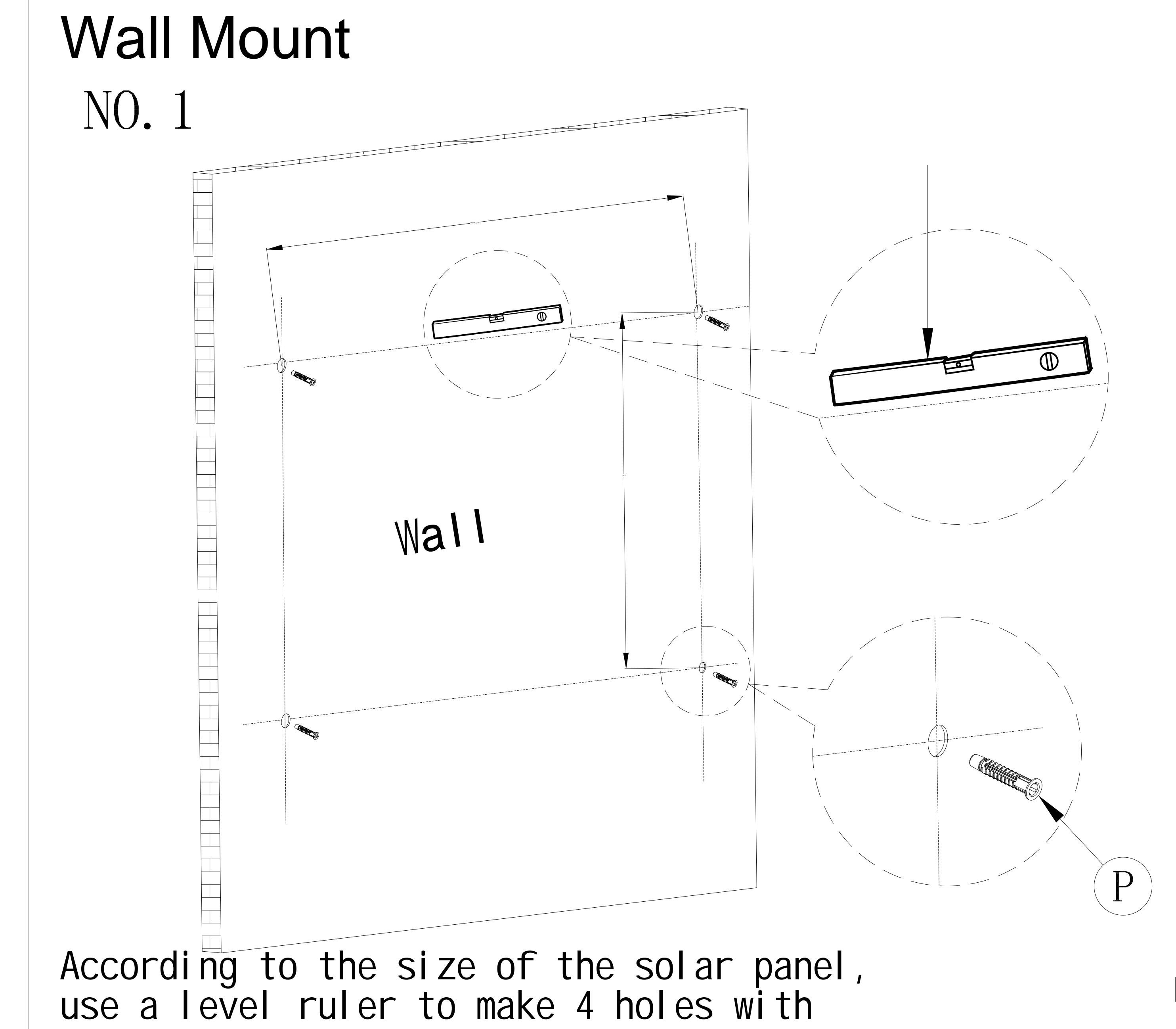
a diameter of 10mm and a depth of 70mm on the wall
