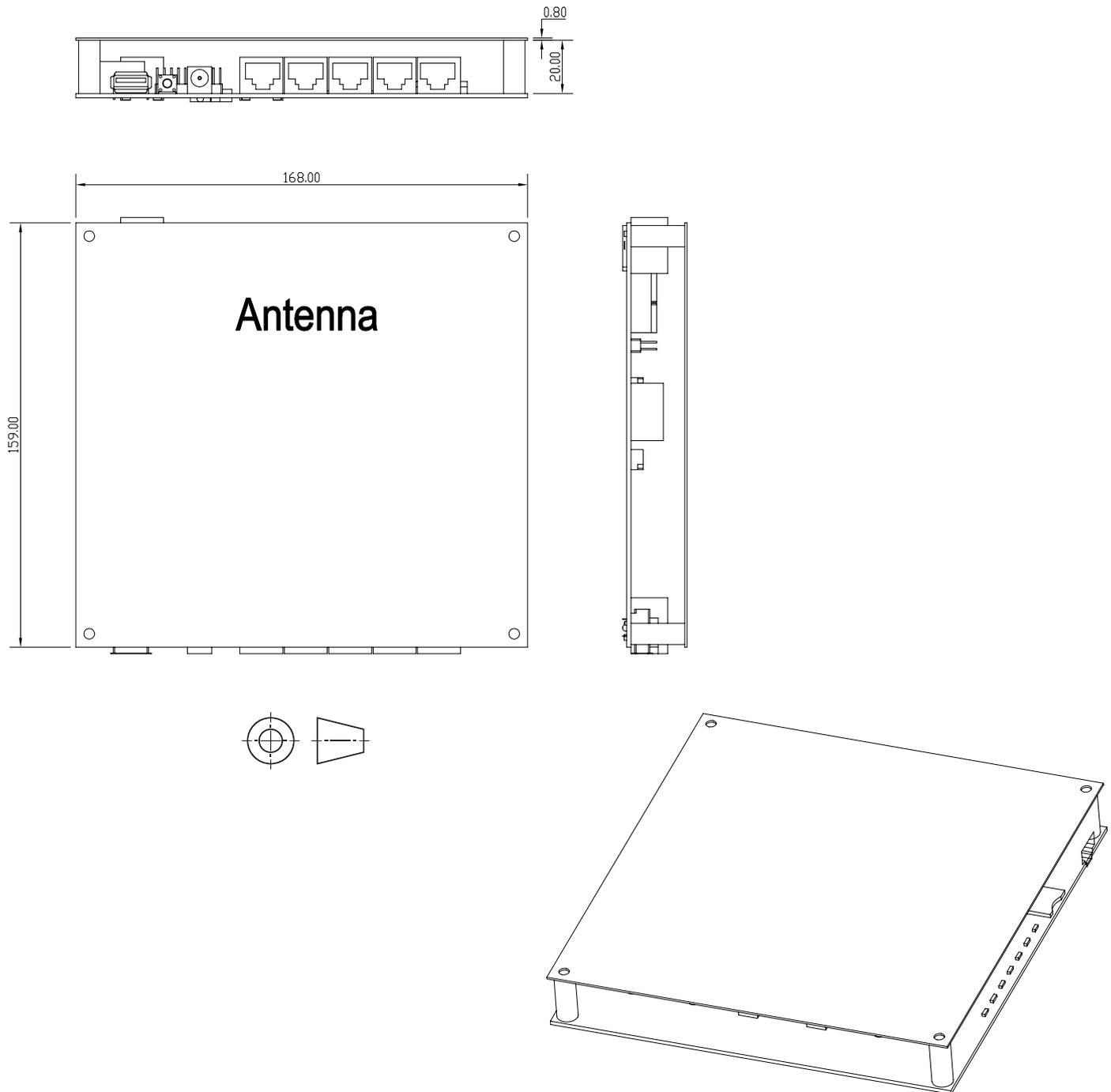
\* The antenna is designed to ride over a host board, which acts as a reflector, as shown in the assembly drawing.
