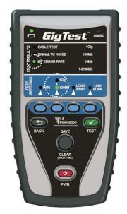
LED indicating pass or fail of BERT test. Will run only if Cable and SNR tests are passed and a second GigTest is at the other end of the cable. This test will show fail if more than 3 errors are detected in the normal length test, or 10 errors in the long length test.
