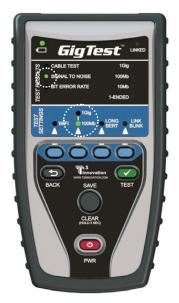
LED indicating pass or fail of the SNR test. Cable must pass Cable Test in order to be run. Will test the 1-2 and 3-6 pairs if 100Mb is selected. All four pairs are tested in 1000Mb mode. SNR is reported if connected to a switch or NIC.
