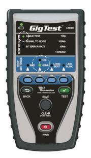
Bicolor LED indicating pass or fail of a cable test. If 10Mb link, cable test only will be run. If 100Mb is selected, only active two pairs are tested. Cable test primarily tests for cable faults that would prevent the possibility of linking, not a complete wire map.
